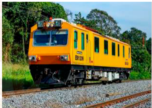
Figure 4. Track inspection Car EM120N [SRT]
