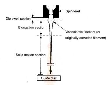
Figure 2.13 The deformation of viscoelastic filament by elongation strain [4]
