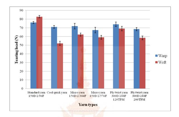
Figure 4.4 Tearing load of fabrics
