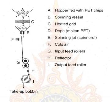
Figure 2.11 Schematic melt spinning process for PET fiber [4]
