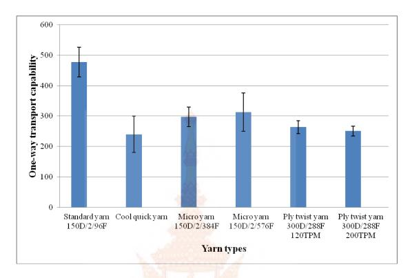
Figure 4.14 Accumulative one-way transport capacity
