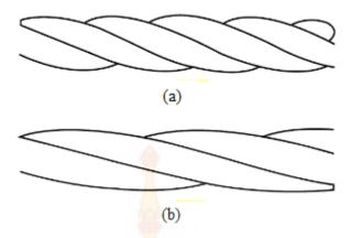
**Figure 4.8** Twisting of the threads (a) high twist (b) low twist [69]
