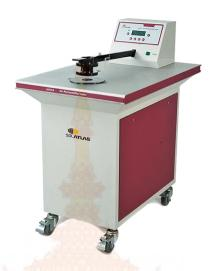
Figure 3.3 The M021A air permeability tester
