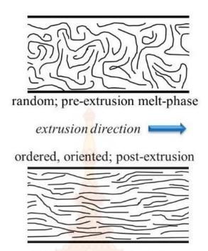
Figure 2.14 The change in polymer chain orientation during the extrusion process[18]
