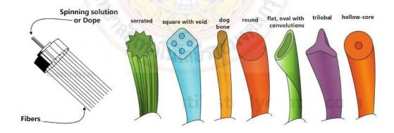
Figure 2.16 Profiled fibers from different spinneret hole [22]
