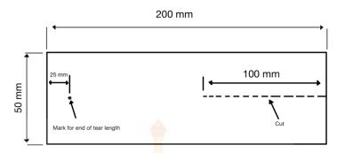
Figure 3.2 Trouser-shaped test specimen
