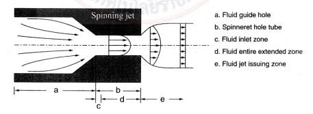
Figure 2.12 The profile model of spinning jet [4]
