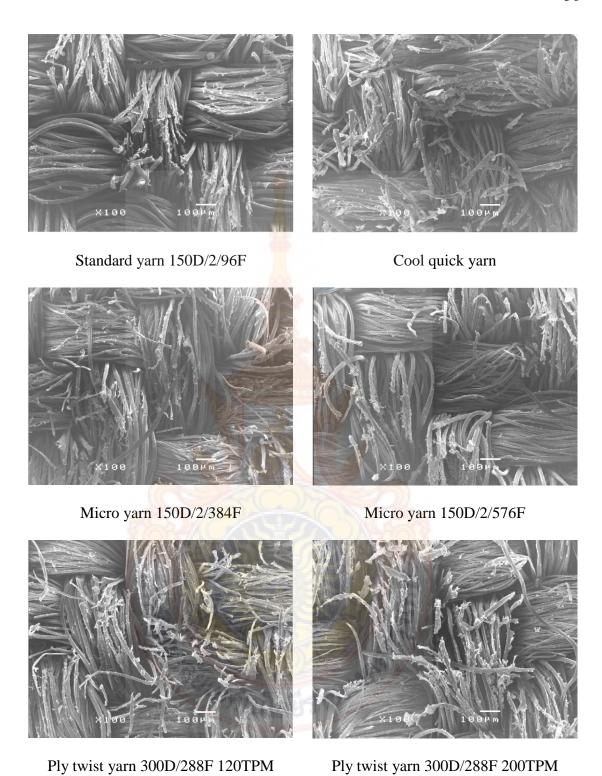
Figure 4.7 SEM micrographs of fabrics after abrasion test
