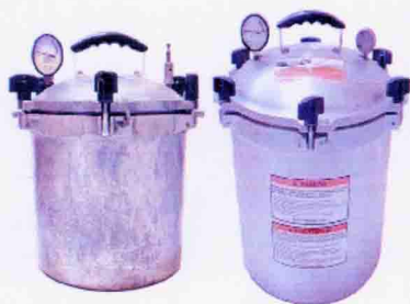
Two stovetop autoclaves
